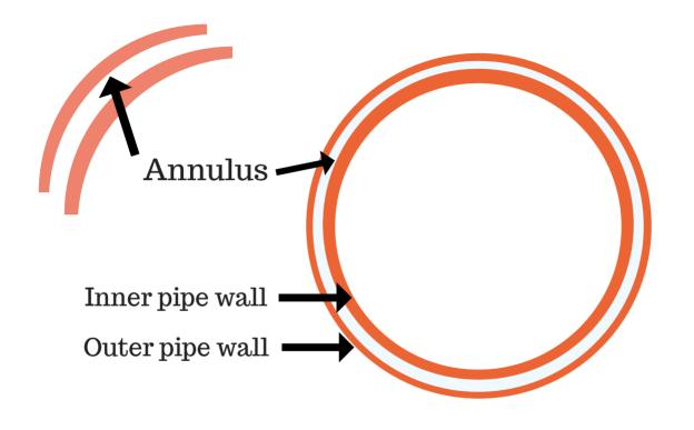
Annulus is the space between the inner pipewall and the outer pipe wall
